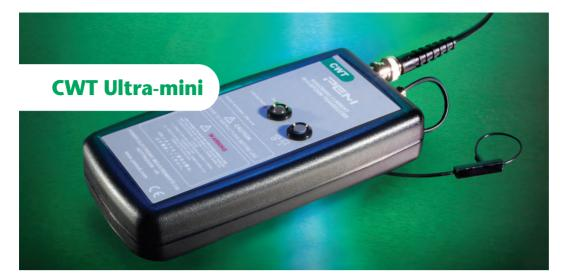
The CWT Ultra-mini has an extremely thin, clip-around Rogowski coil of typically 1.6mm cross-section. Such a thin coil enables currents to be measured in the most difficult to reach parts of a power electronic converter with negligible disruption to the circuit under test.
